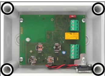
Picture 3 - Wall fixing screw entry points
