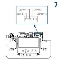
The Loop connector on the top of the translator board should be wired to the Panel of your choice, from the left to right the terminals are:
