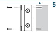
Screw the back box to the wall using all fixing holes and appropriate-sized roundhead screws (do not use countersunk screws).
