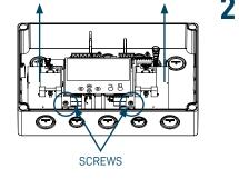
Remove the electronic PCB assembly from the enclosure. The PCB is held by two Philips screws below the display, it then slides up and out.
