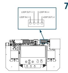
The Loop connector on the top of the translator board should be wired to the Panel of your choice, from the left to right the terminals are:
