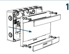
Remove top and bottom front plastics that cover screws, unscrew all four screws and remove the lid from the back box.
