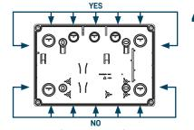
Prepare apertures (20mm knockouts) required for cable access and fit appropriate rated glands.
