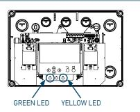
Ensure the LED indicates that the discovery mode is enabled, alternating green and vellow colors.
