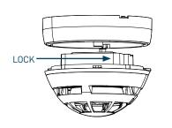
• Ensure you replace the battery cover as this forms part of the detectors anti tamper protection and refit the detector locating it into the base twisting clockwise.
