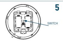
Ensure the programming switch in the base of the detector is in position 1.
