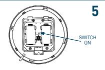
Ensure the programming switch in the base of the detector is in position ON.
