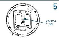
Ensure the programming switch in the base of the detector is in position ON.
