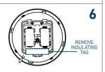
Remove the batteries' insulating tab ensuring the batteries are kept in their lodgement.
