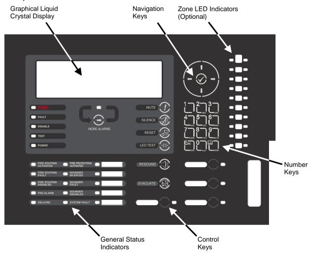
Slide-in labels are used to annotate Function Indicators and Programmable Control Keys and Indicators.
