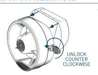
Remove the mounting from the sounder by inserting the security key and turning to the unlocked position on both sides. Pull apart the two pieces.
