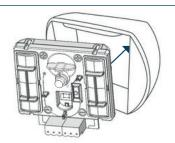
Install the sounder interface module into the base locating the bottom tags and pushing back in.
