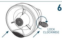
Ensure you replace the battery cover as this forms part of the sounder anti tamper protection.
