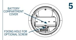
Fit the battery compartment cover on the base.
