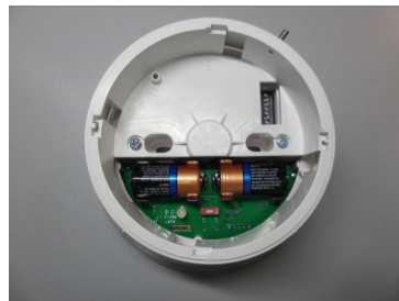
Picture 2 - wireless base sounder top view
