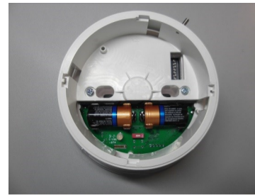
Picture 6 - primary and secondary batteries inserted
