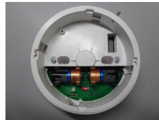
Picture 6 - primary and secondary batteries inserted
