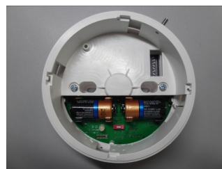
Picture 6 - primary and secondary batteries inserted
