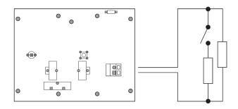
End of line resistor (R $_{\rm eol}$ ) = 5.6K $\Omega$ Alarm resistor (R $_{\rm w}$ ) = 2.2K $\Omega$
