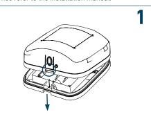
Remove the Wireless Remote Indicator front from the back box pressing the "unlock" button.
