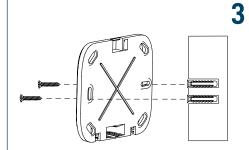
Screw the back box to the wall using all fixing holes and the supplied screws.
